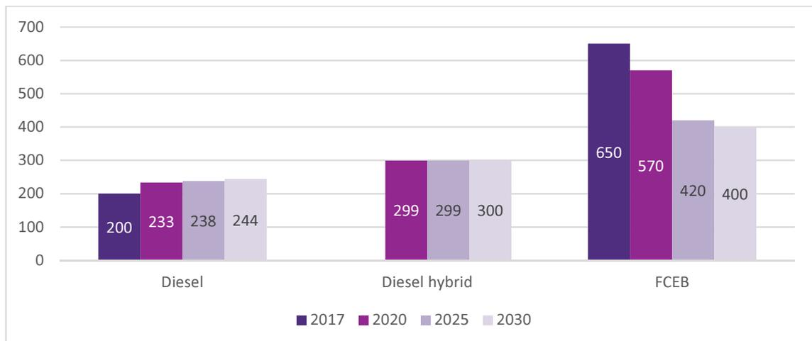
An important parameter for vehicle operators is the total cost of ownership (TCO) which expresses the sum of the acquisition and operating costs expressed per driven km. Figure 8 shows the total cost per kilometre for a Diesel bus, FCEB and FCEB (FCEV FC) with
